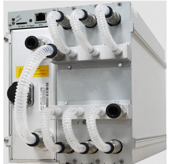
Fig. 1. Bitmain Antminer S21 XP Hydro 473.00 Th/s @ 5676W [4]
